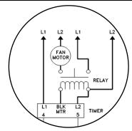
IF DRAFT INDUCER MOTOR IS OVER 4.4 AMPS, WIRE 950-0483 ISOLATION RELAY AS SHOWN IN THIS DIAGRAM.
