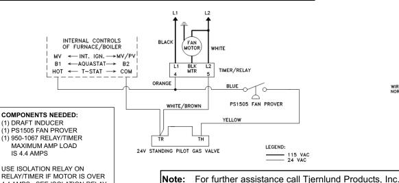
DRAFT INDUCER CONNECTED TO OIL BURNER WITH R8184G CONTROLS (DRAFT INDUCER MOTOR LESS THAN 4.4 AMPS) MODELS I, IL, XL MUST USE 950-0483 ISOLATION RELAY
