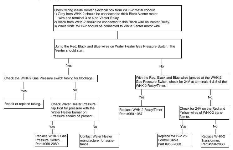
SYMPTOM 3: HSUL, GPAK - SERIES POWER VENTER OR DRAFT INDUCER OPERATES WITH WATER HEATER NOT WITH FURNACE OR BOILER. BEFORE CONTINUING, THE WHK-2 SHOULD HAVE POWER, THE WATER HEATER SHOULD BE OFF AND THE FURNACE OR BOILER SHOULD BE CALLING FOR HEAT.
