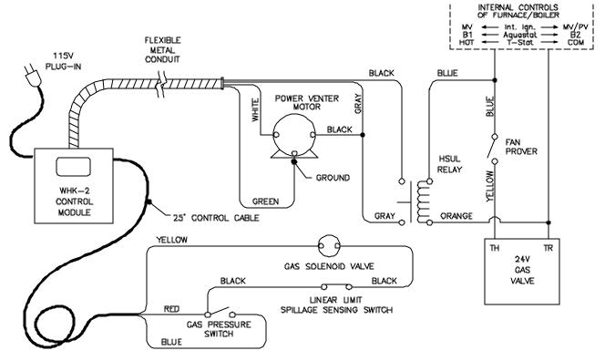
NOTE: THE "HOT" WIRE FROM THE INTERNAL CONTROLS OF APPLIANCE IS THE WIRE NORMALLY CONNECTED TO THE TH TERMINAL OF THE GAS VALVE.
