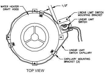
4. Route the Linear Limit spillage switch cable down the water heater casing locating the end near the Solenoid Valve. Secure it with the cable clamps and self drilling screws provided.
