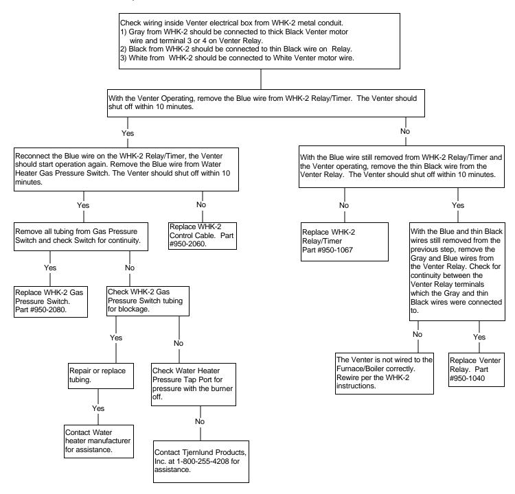
SYMPTOM 2: HSUL, GPAK - SERIES POWER VENTER OR DRAFT INDUCER OPERATES WITH FURNACE OR BOILER NOT WITH WATER HEATER. BEFORE CONTINUING, THE WHK-2 SHOULD HAVE POWER AND THE FURNACE OR BOILER SHOULD NOT BE CALLING FOR HEAT.
