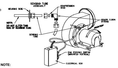
As viewed from the opposite end of the shaft, the motor should rotate clockwise
