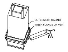
8. Slide the Vent Hood through the wall while taking care installing the rain shield as shown, (See Diagram E). The nuts located on the Vent Hood outermost casing should be facing up when sliding it through the wall. Mount Vent Hood to the exterior using four #8 x 3" wood screws and spacers provided, (See Diagram E). Wall anchors are provided for installation into masonry wall.
