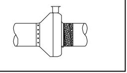
USE SHEET METAL SCREWS (1" MAX) OVER-WRAP WITH DUCT TAPE
