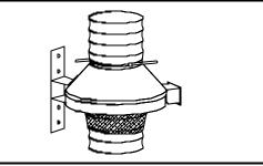
USE NYLON TIES OVER-WRAP WITH DUCT TAPE
