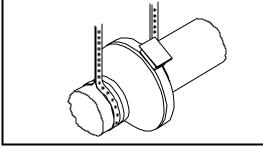
ENCIRCLE WITH PERFORATED PLUMBER'S STRAP & SECURE TIGHTLY CONNECTION WITH FLEX DUCT
