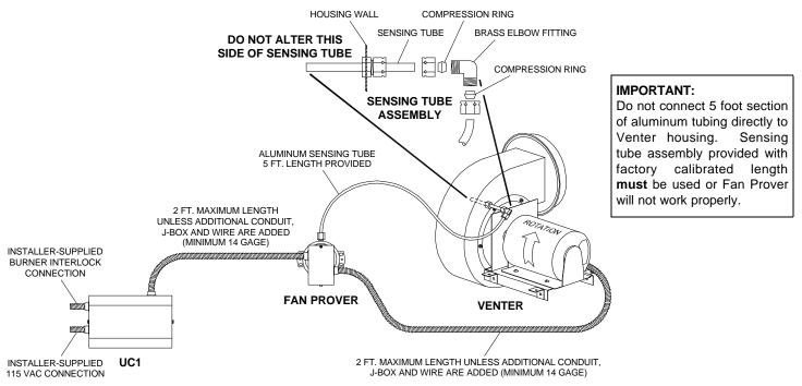
**IMPORTANT:** As viewed from the opposite end of the shaft (rear of motor), the motor should rotate clockwise.
