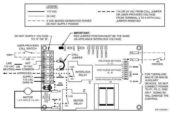
**WARNING:** Disconnect power supply from the UC1 and heating equipment when making wiring connections and servicing the Venter. Failure to do so may result in personal injury and/or equipment damage. LED #5 (RED) should be off with power removed.
