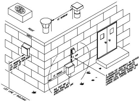
On wall installations, if possible, terminate the Intake Hood on a wall that does not face the direction of prevailing winds. This will diminish the possibility of wind infiltration.
