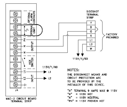
MAC-3 WIRED WITH A POWER VENTER, DRAFT INDUCER OR IN-FORCER WITH A MOTOR GREATER THAN 9 AMPS TJERNLUND MODELS INCLUDE THE XL DRAFT INDUCER, HS-5 POWER VENTER & PAI-7 IN-FORCER
