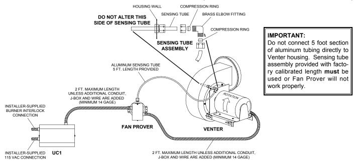
**IMPORTANT:** As viewed from the opposite end of the shaft (rear of motor), the motor should rotate clockwise.
