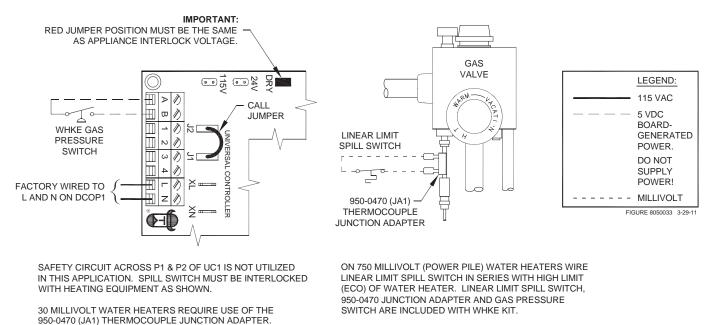
Each millivolt appliance interlocked with the UC1 must have its own WHKE kit installed. The WHKE Gas Pressure Switch actuates the Inducer through the A - B Dry contacts. The Linear Limit switch disables the heater in the event of a venting malfunction.
