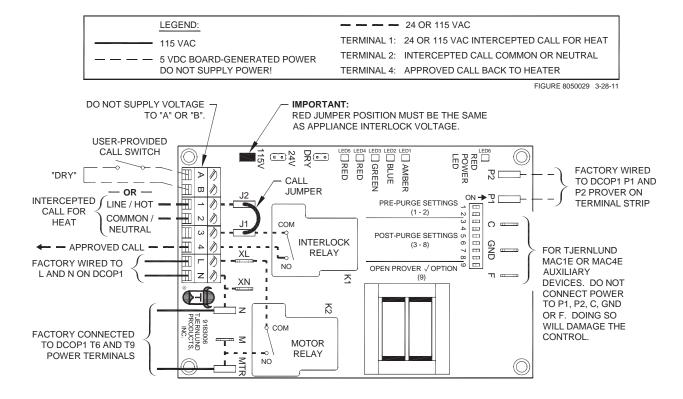
**WARNING:** Disconnect power supply from the DCOP1 and heating equipment when making wiring connections and servicing the Inducer. Failure to do so may result in personal injury and/or equipment damage. LED #6 (RED) should be off with power removed.
