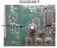
REMOVE #4 WIRE FROM UC1, MAC1E OR MAC4E CONTROL. ON MILLIVOLT APPLIANCES TURN THER-MOSTAT OFF.
