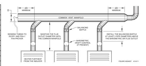
**Example:** A vent layout is required for a job that consists of 4 heating appliances. 1 Appliance has an 8" diameter vent connector, 2 appliances have 6" diameter vent connectors and 1 appliance has a 4" diameter vent connector.
