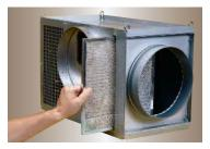
The IN-FORCER attaches with integral mounting brackets or "eye" bolts. The inlet/outlet collars are 2 1/4 inches deep for easy duct connection. The IN-FORCER features a blower that slides out for easy servicing and a washable aluminum mesh pre-filter.
